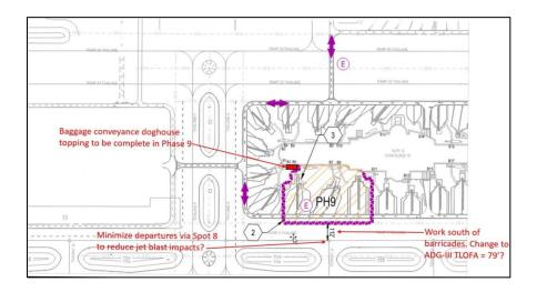
The work area will be surrounded by interlocking, low-profile barricades. ARFF routes will be provided with gaps in the barricade. Pedestrians and vehicle traffic are to stay outside of the barricade during the closure.
