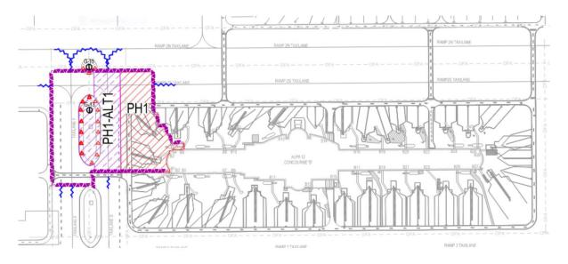
The work area will be surrounded by interlocking, low-profile barricades. ARFF routes will be provided with gaps in the barricade.
