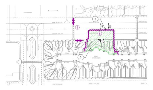
The work area will be surrounded by interlocking, low-profile barricades. ARFF routes will be provided with gaps in the barricade.
