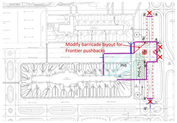
The work area will be surrounded by interlocking, low-profile barricades. ARFF routes will be provided with gaps in the barricade.
